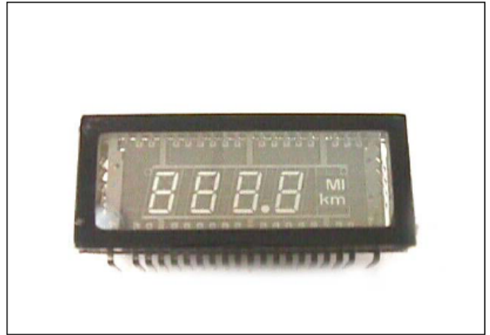
Fractured VFD display. Note the white spot in lower left corner.
