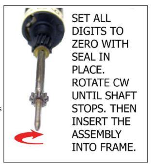
groove at the bottom of the frame. Do not force the assembly into its location as you might break the seal if it is not done carefully.
