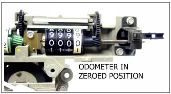
Now that once the retainer is repositioned, the trip odometer wheels will be slightly moved to the right. However, it will still be fully visible in the window cut into the dash faceplate. The difference in alignment is the 1/32" shift on the position of the locking washer stop.
