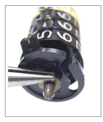
Very carefully remove each part of the assembly, being extra careful to keep the order in which the parts are assembled. The metal plate between each number wheel has a small gear placed into a slot on the plate. This gear must be kept in its original place and can't be reversed on the plate, so take note as to how the gear is positioned on the plate.
