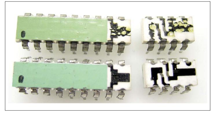
The repair and recalibration involves replacing both network chips, then recalibrating both the boost and tach sections of the module on the bench using a calibration standard. The calibration is performed using a diamond cutting tool instead of a laser, since the diamond tool doesn't exhibit extreme heat in the region of the resistor pad. The chips are then fully sealed with a coating after the calibration process.
